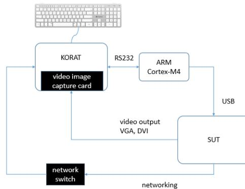
Fig. 4. KORAT Capture/Replay architecture with keyboard.
